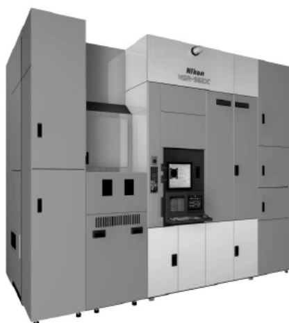
Figure 1. a) High-end “factory application” for 45 nm device production (Nikon NSR610C ArF Immersion Scanner) versus b) a simple “field application” for car refinish in a body shop (Akzo Nobel NV)
